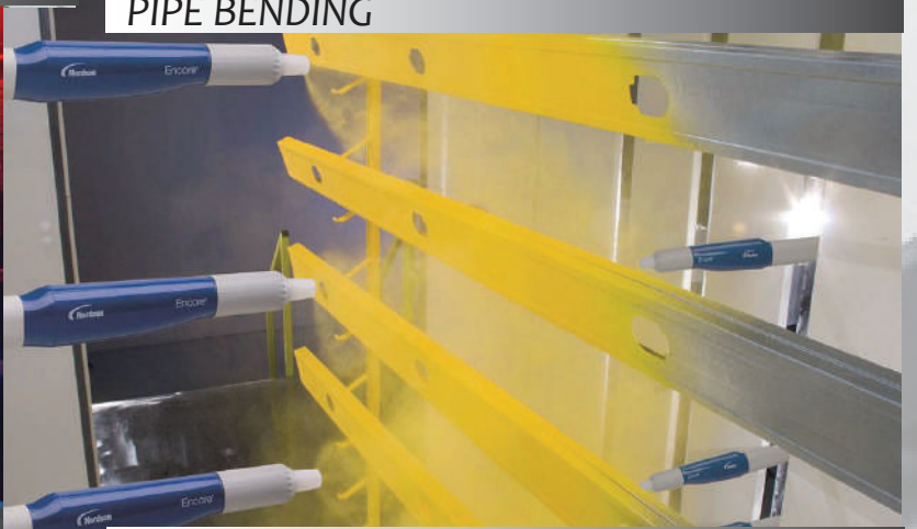
AUTOMATED POWDER COATING
